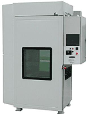
**HASS** - Highly Accelerated Stress Screening is used to find defects and flaws in production to monitor the quality and consistency of your manufacturing processes.
